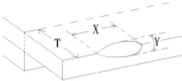
$\Phi = (x+y)/2 > 2.5 \text{ mm}$<br>Reject                                                                                                                |
